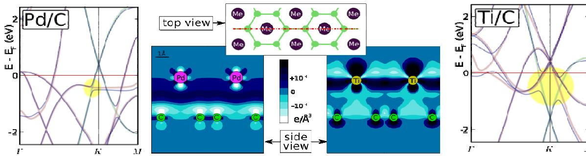
*Pd binds weaker than Ti but allows for better transmission...*
