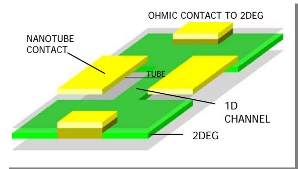
**F.006: Charge transport in CNT driven by surface acoustic waves**
