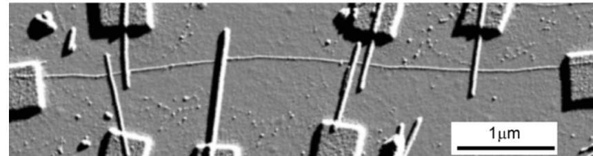
Using MWNTs as noninvasive voltage probes in 4p measurements : intrinsic resistance & observation of negative four-terminal resistance at He temperature
