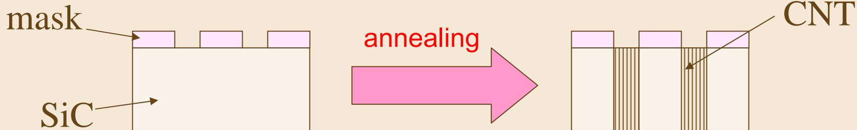
We used Ti as a mask for selective growth of CNT on SiC, since the melting point of Ti is higher than the decomposition temperature of SiC surface.
