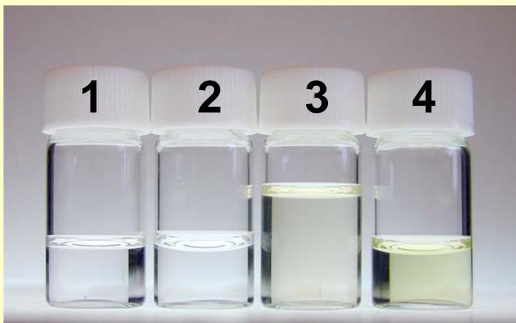
Sample 1: saturated solution of C<sub>60</sub> in THF
