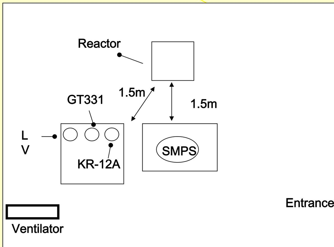
**SMPS :Scanning mobility particle sizer (TSI Model 3034)**
